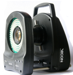
Image 1: The LED strobe lights visible of the Vicon MX3+ camera. These strobes emit light while the camera records its reflection of the white reflective markers worn by the subject. As can be seen, the camera is very portable and is able to be mounted on either a tripod or wall mount. Images courtesy of http://www.vicon.com . 27 March 2007
