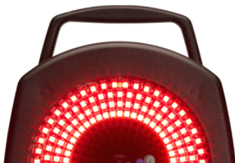
Image 1: The LED strobe lights visible of the Vicon MX3+ camera. These strobes emit light while the camera records its reflection of the white reflective markers worn by the subject. As can be seen, the camera is very portable and is able to be mounted on either a tripod or wall mount. Images courtesy of http://www.vicon.com . 27 March 2007
