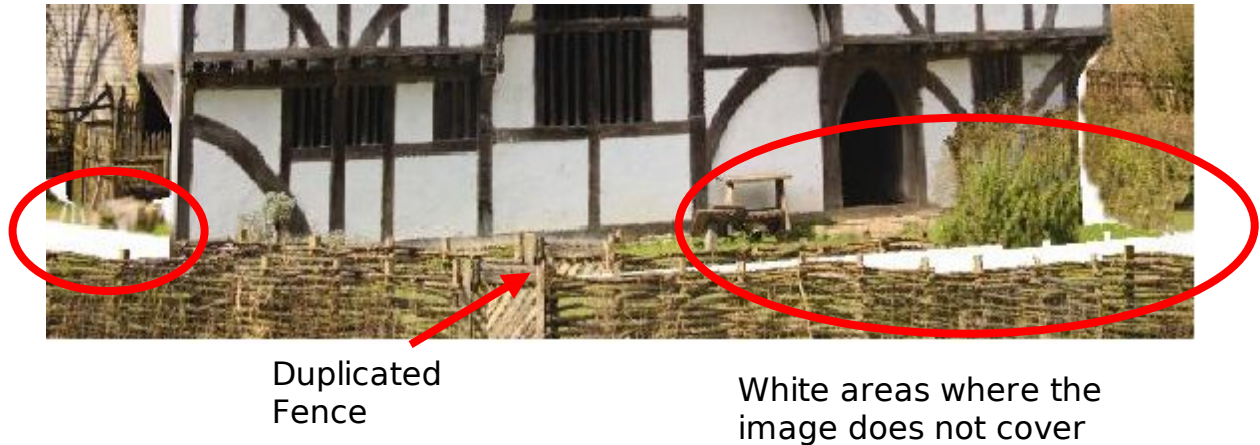
(fig. 14) – Errors with the Projection Map
