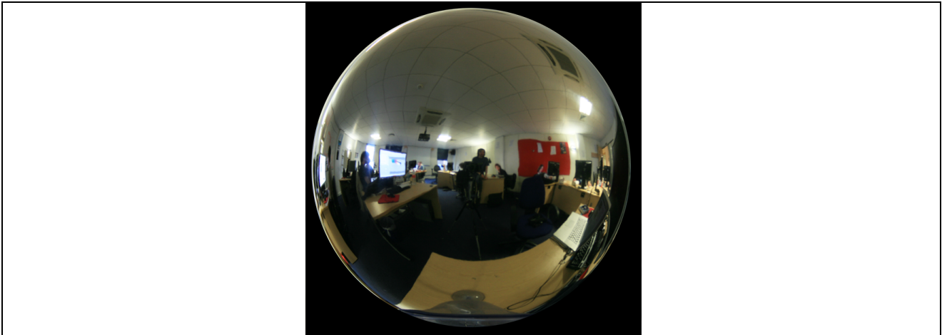
Figure 5, showing a mirrored ball can be used as a light probe. The probe acts as an extream fish eye, covering 360.
