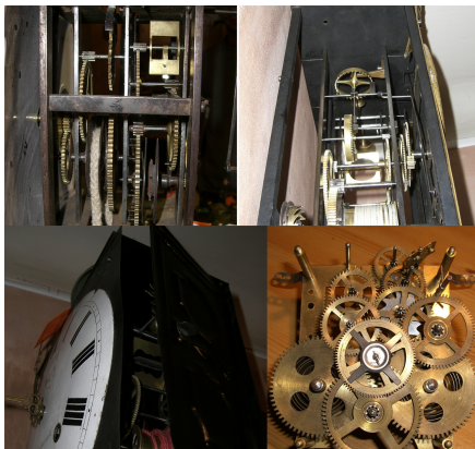
Mechanisms mainly consist of spur gears
