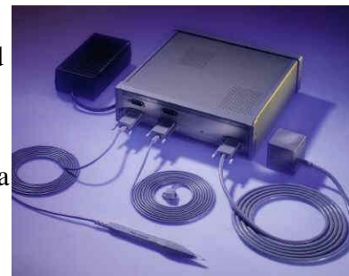
Figure1 "Polhemus Fastrack stylus and sensor" from Inition www.inition.co.uk
