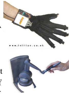
Figure 2 “Dataglove (top) and force feedback armature (bottom)
