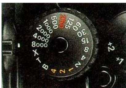
Fig 11: An example of a shutter speed dial. The values in yellow refer to full seconds whereas the numbers in white refer to fractions of a second. The number in red indicates this is the cameras flash sync value. (Source: http://jrp.nikonians-images.com/f4_images/shutter_speed_dial.jpg accessed 5 th March 2006)
