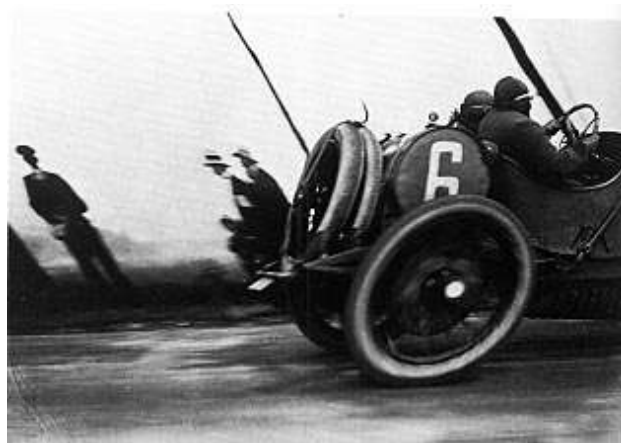
Fig 15: A photo taken with a camera that has a vertical shutter. The shutter starts at the bottom and moves upwards. As the car is moving perpendicular to the shutter (left to right in the image), it makes the car image (and especially the wheel) slant in the direction of its motion. From the way the people in the background are slanted, you can tell the photographer was panning the camera to follow the car. Also, from the minimal blur visible in the image, it is apparent that a fast shutter speed was used. Photograph by Jacques-Henri Lartigues.
