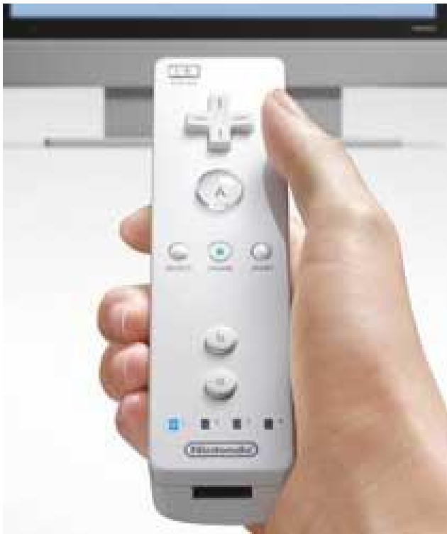
Nintendo “Revolution Controller” (as yet unreleased): Simply by pointing and moving the controller in space will possibly directly control the game accordingly, with the aim being intuitive control. Thus the need for instruction manuals is decreased, a whole possibility of new game genres is created, with the increased intuition acting as connection to people who don’t generally play computer games.
