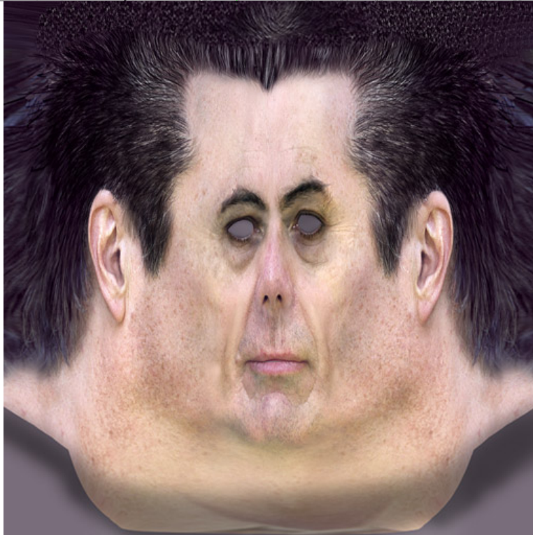
Cylindrical map with distortion at the top and bottom Example of a predistorted game texture from half-life 2
