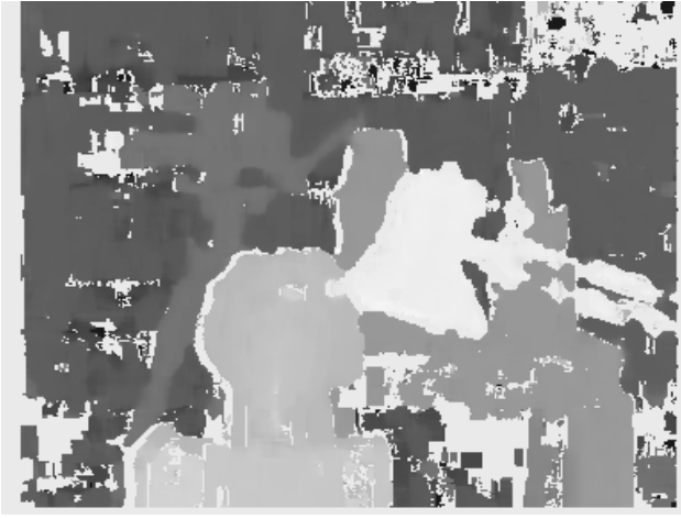
Fig. 9. Disparity map of the "tsukuba" image pair for a window size of 7 \times 7 pixels. Pixels that were rejected by the left-right or uniqueness test are shown in yellow.
