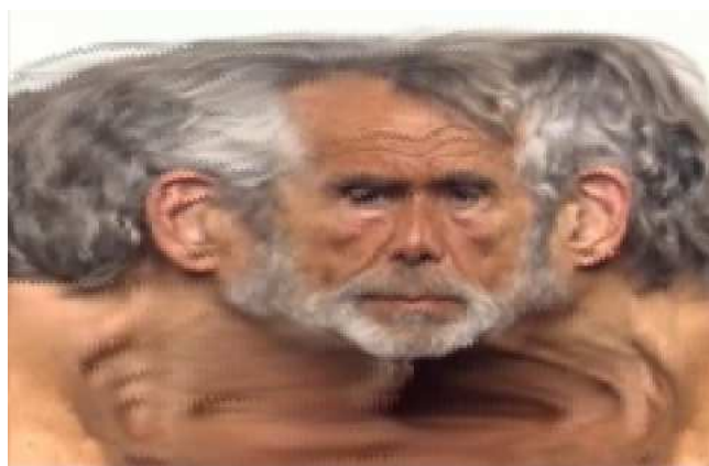
Figure 12 A Cylindrical map is generated by placing the subject on a turntable. Source: The Human Motion Show
