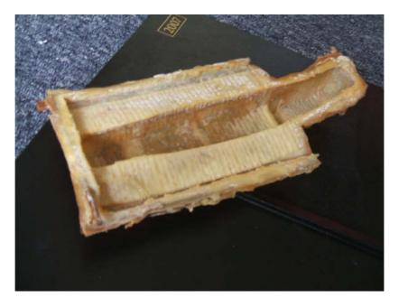
It took several layers of liquid latex to make the mould thick enough to hold its shape. This mould was for the brick columns and part of the walls either side of it. Despite its thickness, it was quite wobbly and I had to be careful to make sure the edges were straight when I used it to cast more columns.
