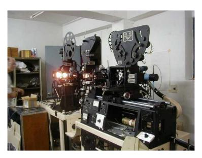
Optical Printers are incredibly complex machines that consist of a projector (able to project double-thickness film to allow for layering with the mattes) linked to a film camera, to copy footage from one filmstrip to another. (*Ref* 8).
