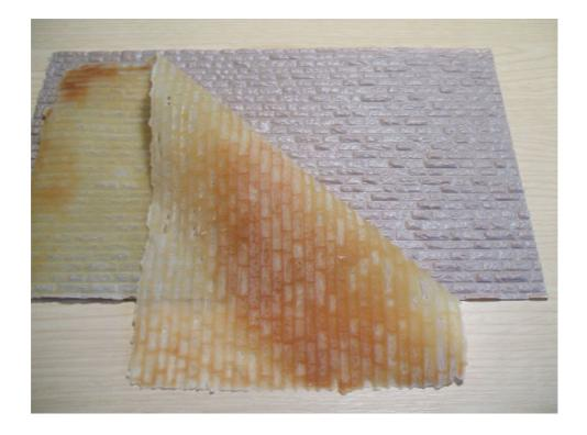
I used this latex mould to cast many flat sheets of plaster, each typically 5mm thick, and all with the detailed brick texture on. They were easy enough to cut, although they did tend to break quite easily, and I found the PVA glue stuck them together well.
